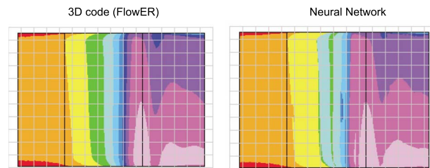
Fig. 3 A comparison of enthalpy distribution predicted using ANN and calculated by the FlowER solver at the axial section at 62% of the rotor blade channel
